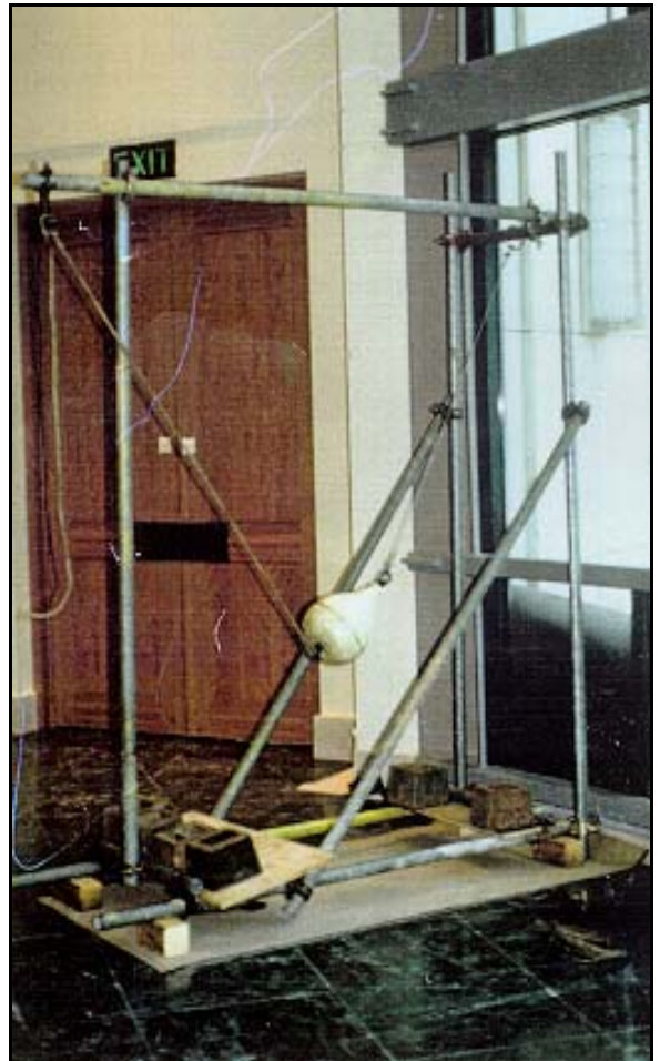
Photograph showing testing equipment, including Impactor Ball, for testing glass panel
