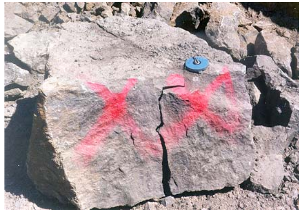
Failure of a rock armour unit during rough handling, leading to rejection
