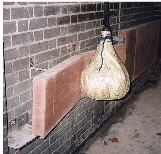
Soft body impact test
